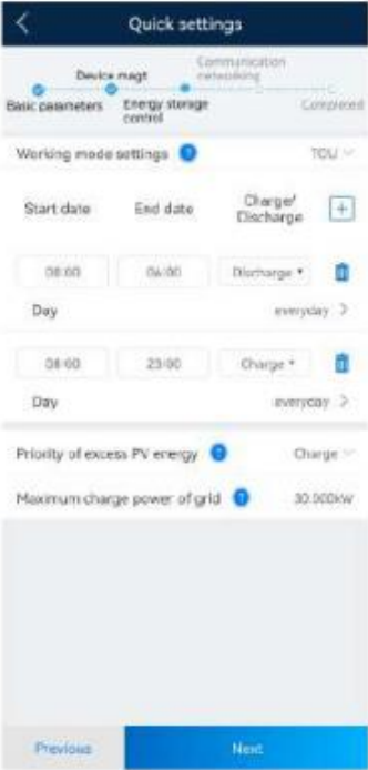
Figure 4-7 TOU (time-of-use) working mode
