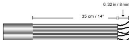
Figure 28: Insulation stripping – AC
